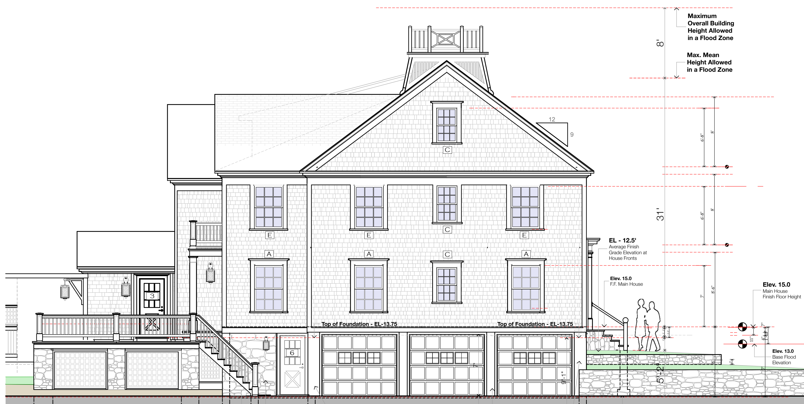
3 LEFT SIDE (EAST) ELEVATION 3/16" = 1'-0"
