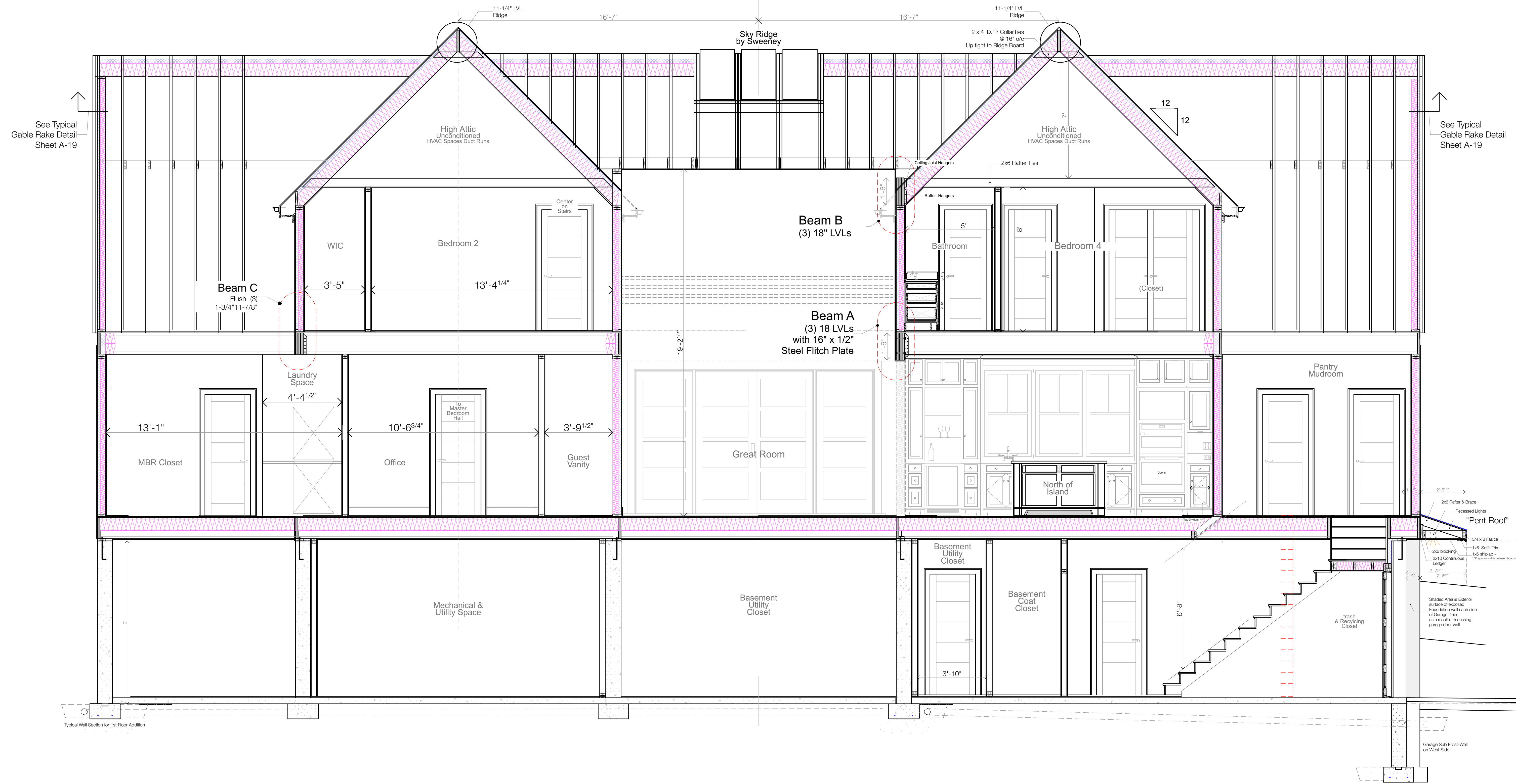
Long Section Thru - MBR Hall, Great Room, Dining Room, Pantry Mudroom and Corner Stairs
