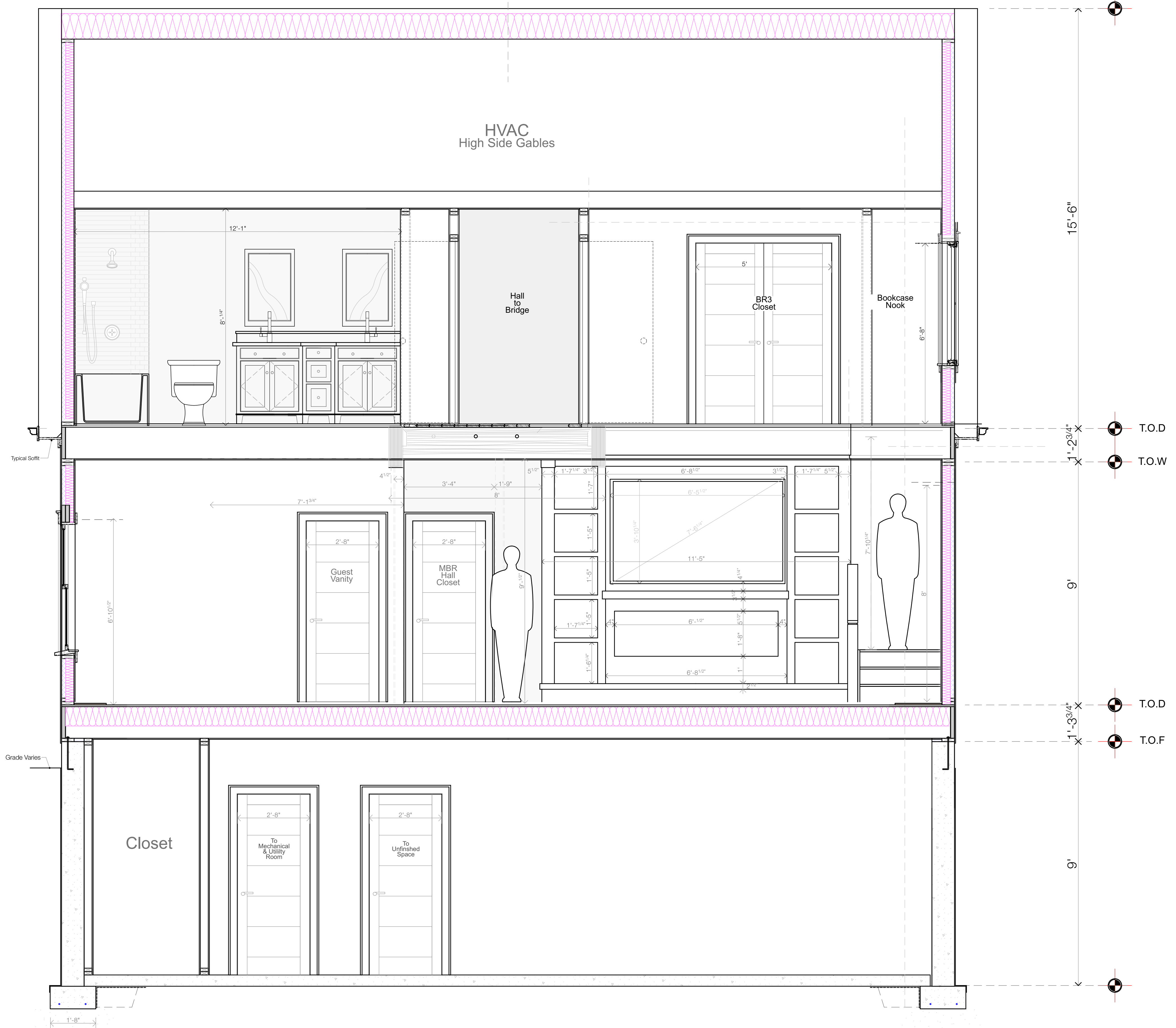
Section 5 - Dining Room and Kitchen - Looking East Before Cabinets Begin
