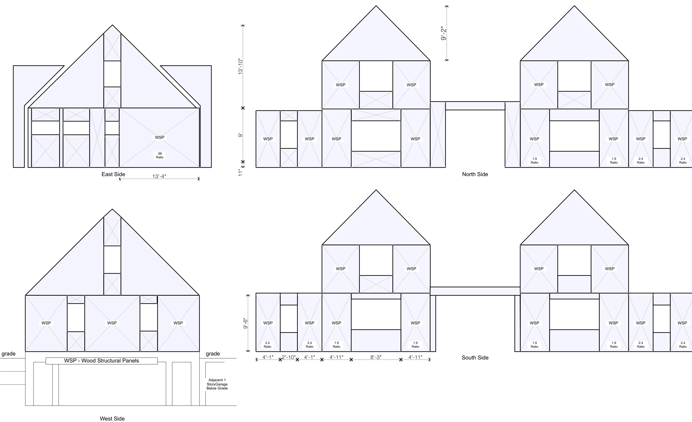
Lateral Bracing Exterior Walls
